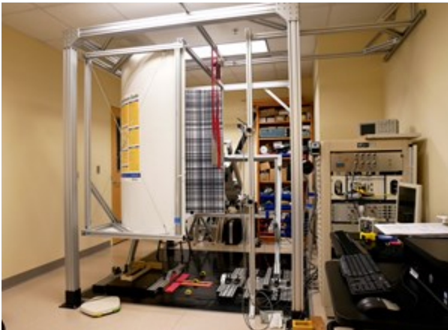
Figure 1. NCRAR custom balance test device. Test subjects stand or step in place while facing the plaid pattern of the visual surround. Balance is perturbed by rotation of the visual surround or the stance surface. Body sway motions, surface forces, and foot placement are measured and related to the perturbing stimulus to assess balance control behavior.
